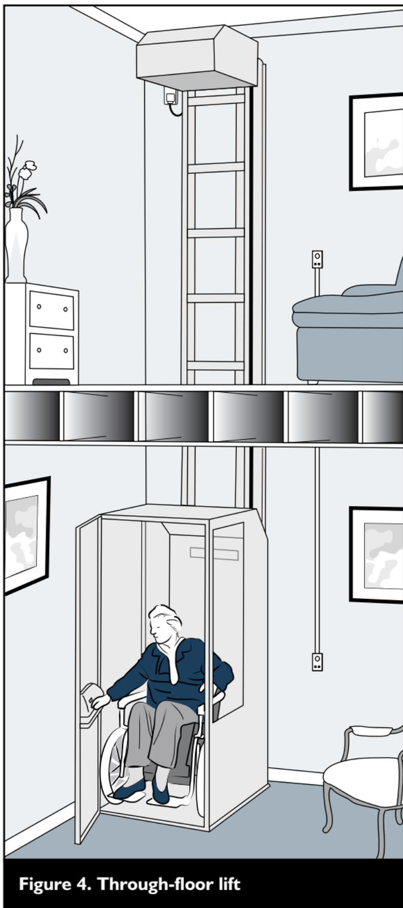
**Figure 4. Through-floor lift**
