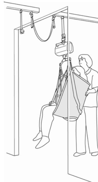
Running ceiling track through from one room to another can involve costly alterations that may not always be structurally possible. Some companies offer a solution that enables the user plus lifting unit to be transferred onto track on the adjacent side of a door header using suspension straps.
